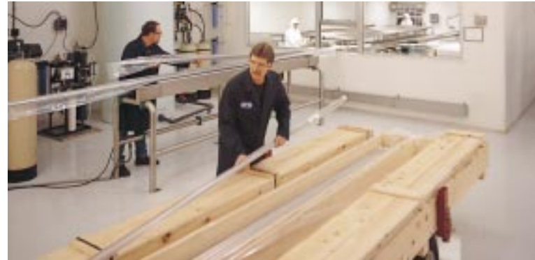
Rath's certified Class 100 Cleanroom is where electropolished tubing receives 100% inspection, final cleaning and packaging.
